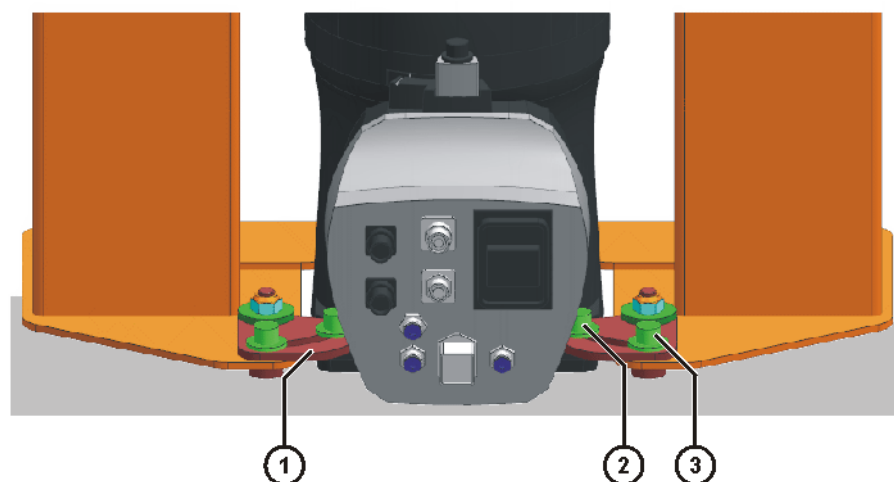
Fig. 8-5: Positioning and fastening the swivel holders
